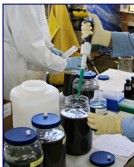
Researcher demonstrates the new method for spiking nickel into sediments
